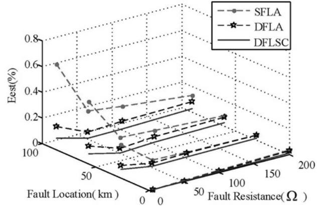
**Fig. 7** Estimate errors of three algorithms under ABC fault with different fault resistances at different distances
