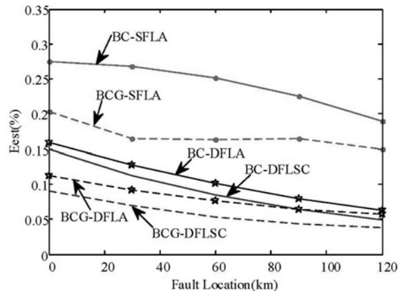
**Fig. 12** Mean errors of fault location estimate of three algorithms under different fault types and different distances, when the fault resistance is 100 Ω
