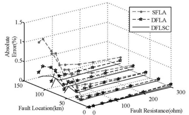
**Fig. 8** Absolute errors of three algorithms under ABC fault with different resistances at different distances
