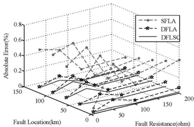
**Fig. 10** Absolute errors of three algorithms under ABC fault with different resistances at different distances
