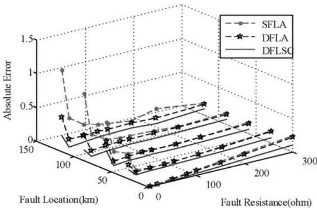
**Fig. 6** Absolute errors of three algorithms under ABC-G fault with different fault resistances at different distances
