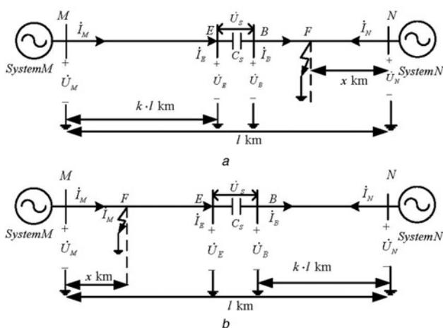
**Fig. 1** Circuit diagrams of series-compensated transmission line with a fault on the
