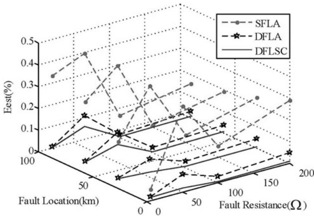
**Fig. 9** Mean errors of three algorithms under ABC fault with different fault resistances at different distances
