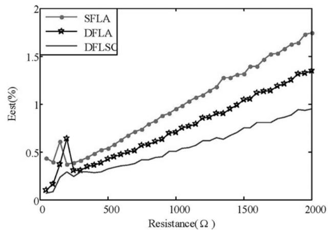
**Fig. 11** Mean errors of three algorithms under A-G fault with different resistances when the fault location is 60 km
