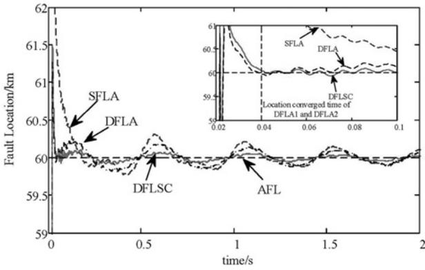
**Fig. 5** Fault location estimate of three algorithms under an ABC-G fault (fault resistance: 100 Ω; fault distance: 60 km)
