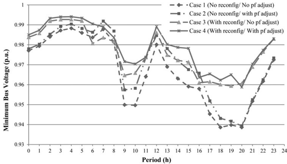
Fig. 6 Minimum bus voltage observed for every hour of a day for all cases for 10% increased load
