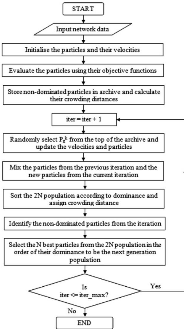
Fig. 3 Flowchart of the proposed method for implementation of NSPSO for network reconfiguration
