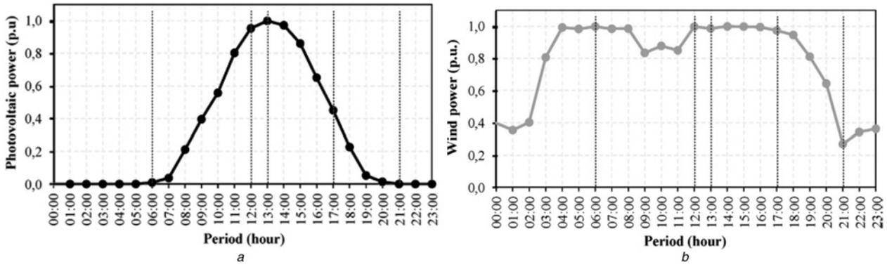
Fig. 2 Normalised DG generation curve [1]
