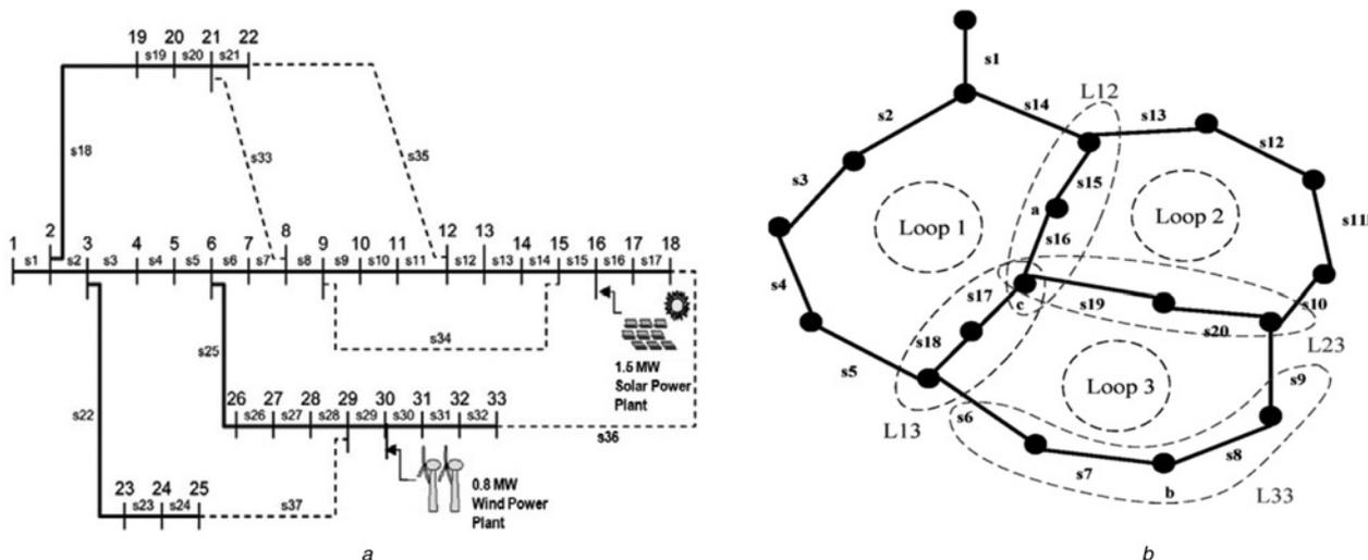
**Fig. 4** Single line diagram of IEEE 33-bus and its sample network
