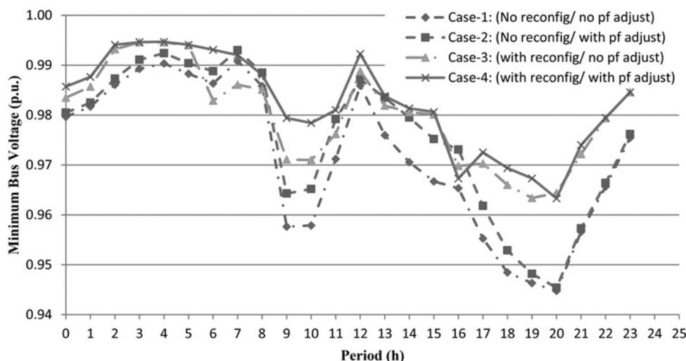
**Fig. 5** Minimum bus voltage observed for every hour of a day for all cases for nominal loading
