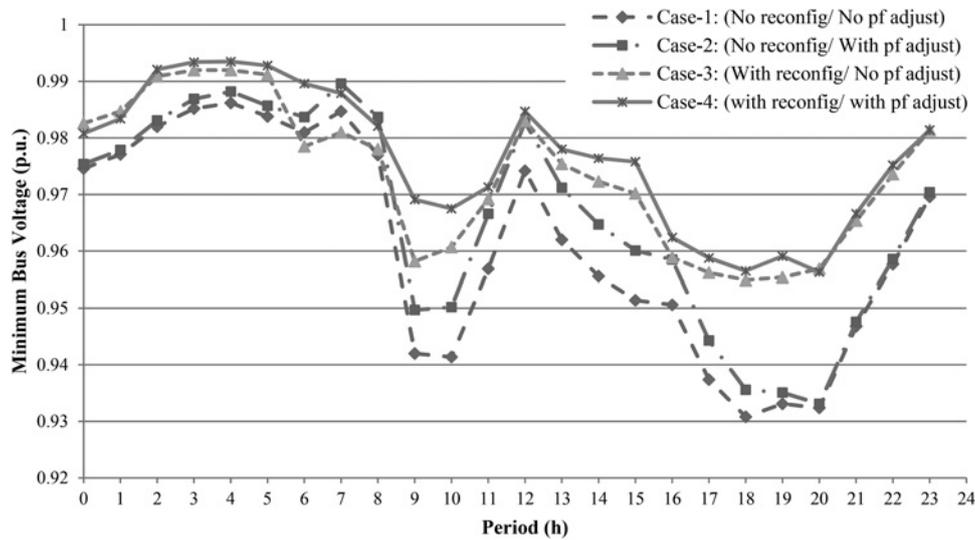
Fig. 7 Minimum bus voltage observed for every hour of a day for all cases for 20% increased load
