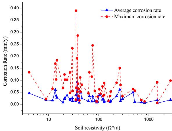
Figure 6. The relationship between soil resistivity and substation grounding grid corrosion
