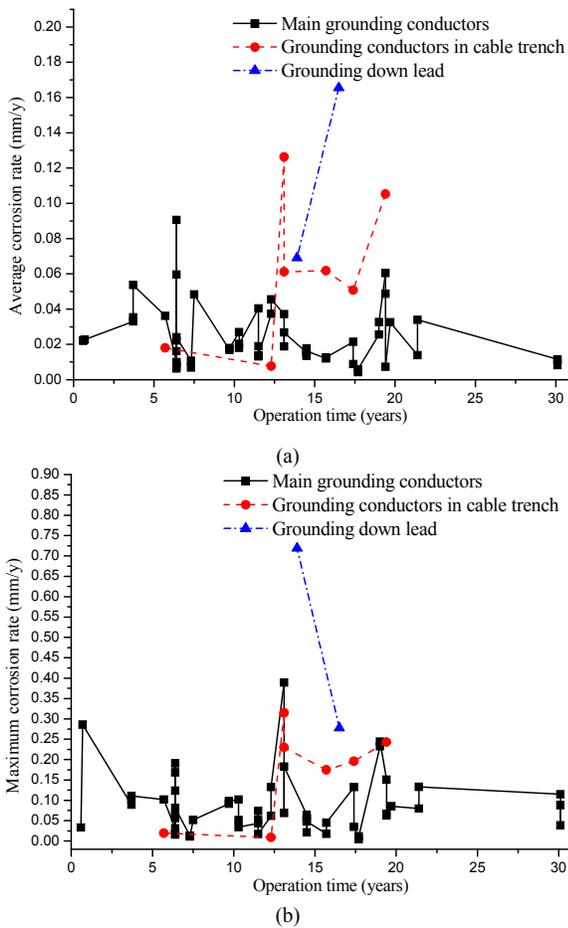
Figure 5. The relationship between the substation grounding grid corrosion and operation time for (a) average corrosion rate and (b) maximum corrosion rate
