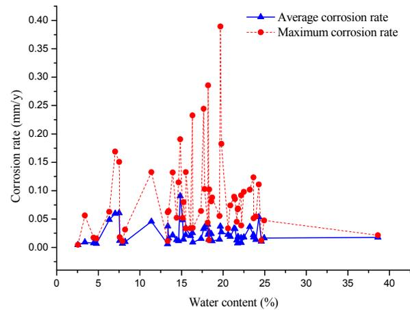
Figure 8. The relationship between water content and substation grounding grid corrosion
