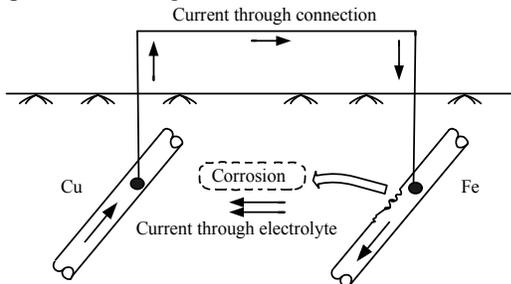
Figure 2. Galvanic corrosion
