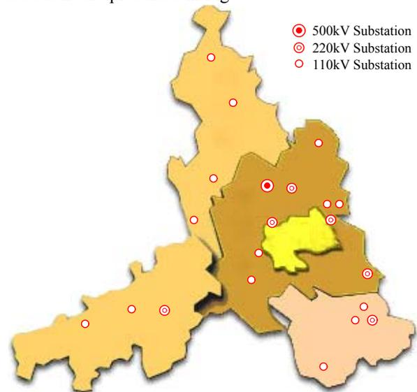
Figure 4. Distribution map of sampled substations in Foshan area
