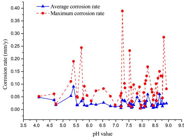
Figure 7. The relationship between pH value and substation grounding grid corrosion
