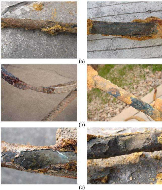
Figure 3. Corrosion forms of (a) uniform corrosion, (b) pitting corrosion and (c) microbial influenced corrosion in substation grounding grid
