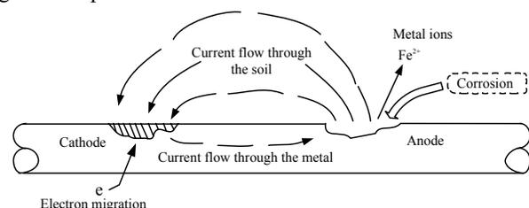
Figure 1. A basic galvanic corrosion cell
