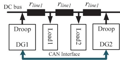
Fig. 2. Distributed dc microgrid.
