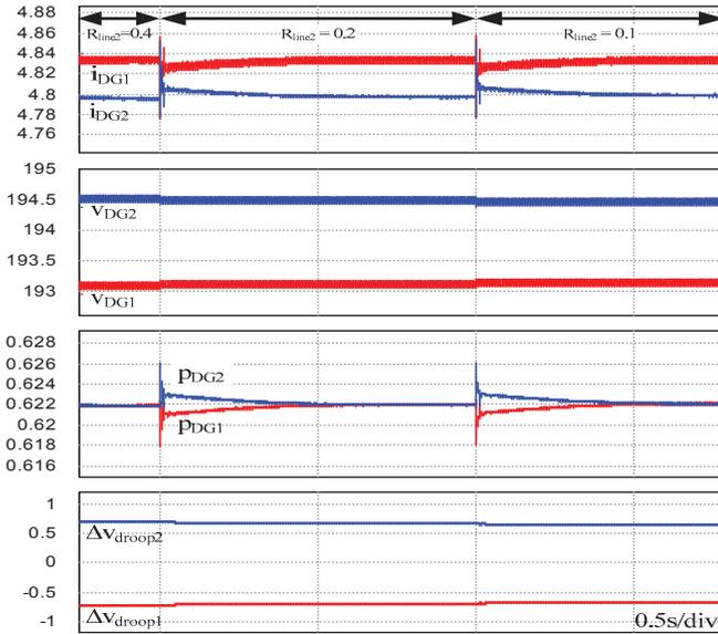
Fig. 10. Proposed method with changes of equivalent line impedance.
