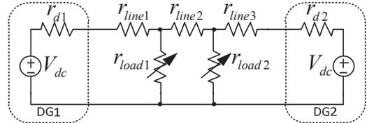
Fig. 3. Equivalent circuit of a dc microgrid with two DGs and two loads.
