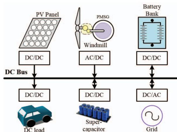
Fig. 1. Typical configuration of dc microgrid.
