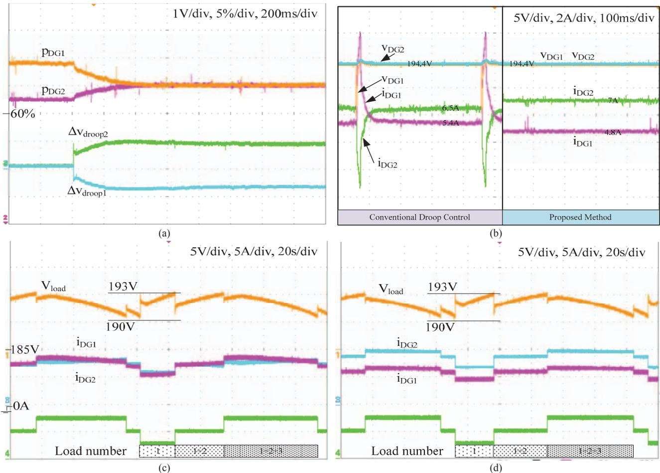
Fig. 13. Experimental results (a) Transient of proposed method (b) performance of conventional and proposed method (c) load shedding with conventional droop control (d) load shedding with proposed method.
