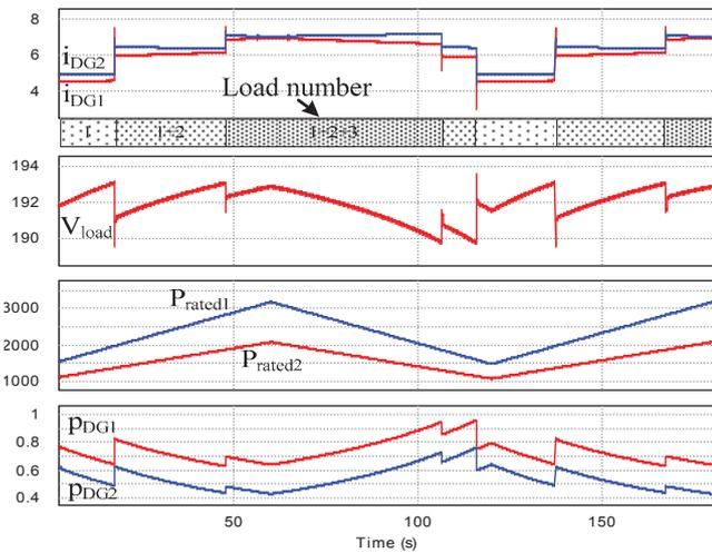
Fig. 11. Load shedding with conventional droop control.
