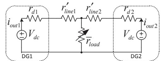
Fig. 4. Equivalent line impedance and equivalent load.
