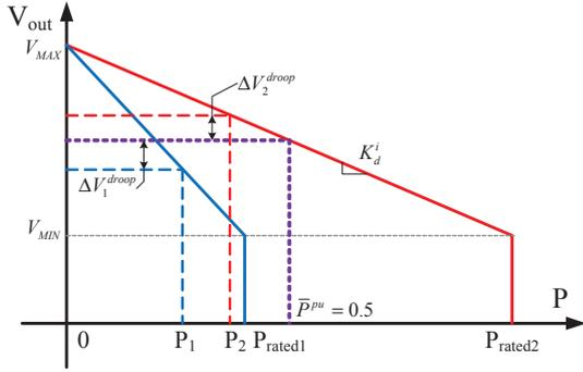
Fig. 8. Droop characteristics for each DGs with difference of power rated.
