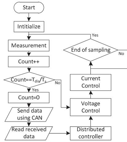
Fig. 5. Flowchart of proposed control scheme.
