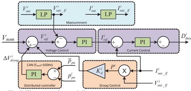
Fig. 7. The proposed control diagram.
