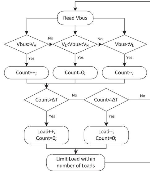
Fig. 6. Flowchart of load shedding procedure
